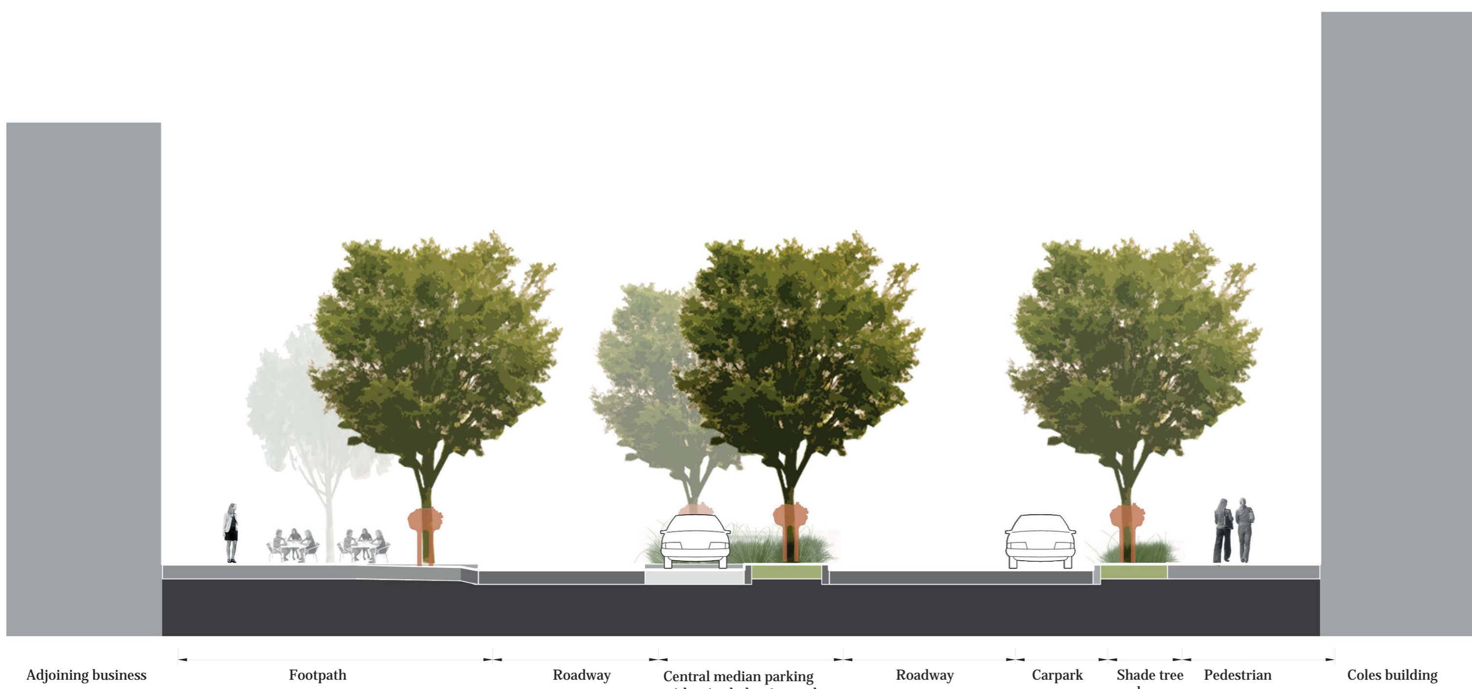
Section BB Central median with raised planting
