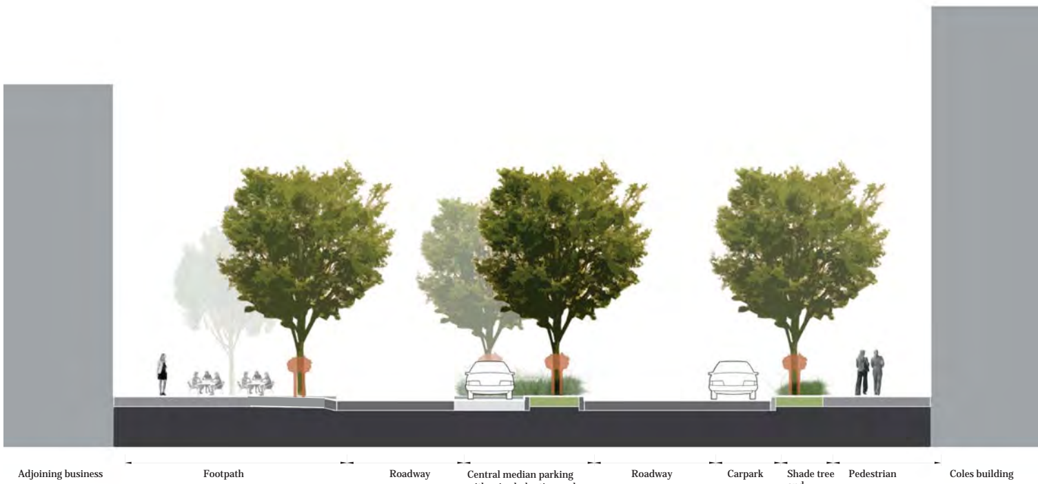
Section BB Central median with raised planting
