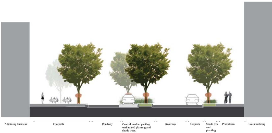
Section BB Central median with raised planting
