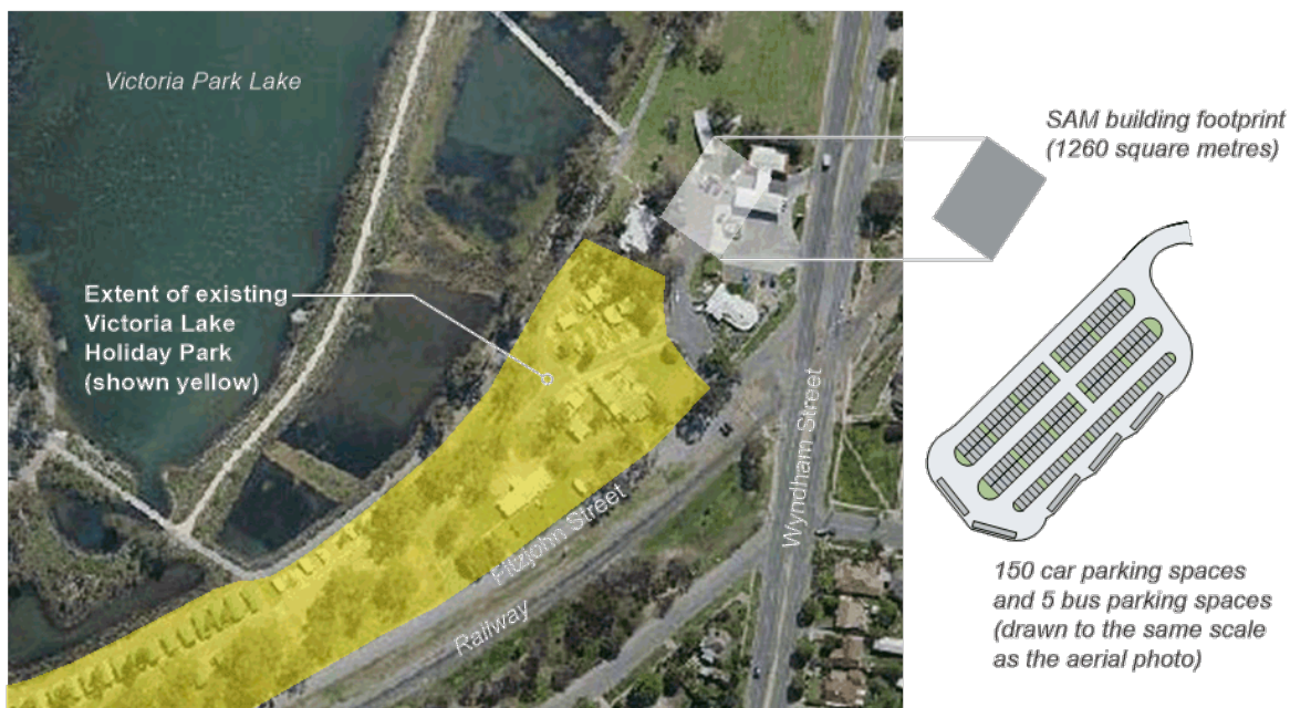
Figure 6 A comparison in size between the SAM building footprint, and the area required to accommodate 150 car parking spaces and 5 bus parking spaces.
