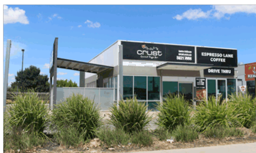
Encourage: Muted colours and tonings, large window proportions oriented towards the streetscape and use of verandahs to minimise visual bulk
