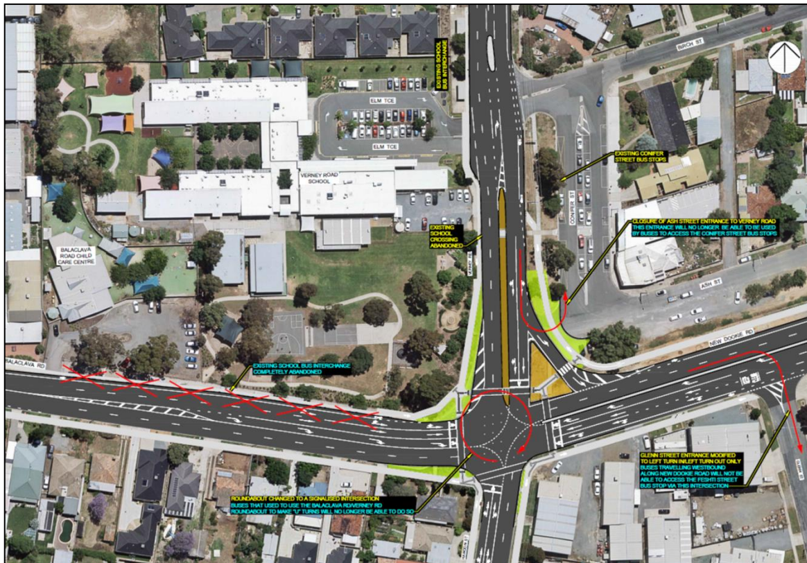
Figure One: Ultimate Balaclava Road – Hawdon Street – New Dookie Road – Verney Road Intersection. The existing Balaclava Road School Bus Interchange is identified with red crosses.
