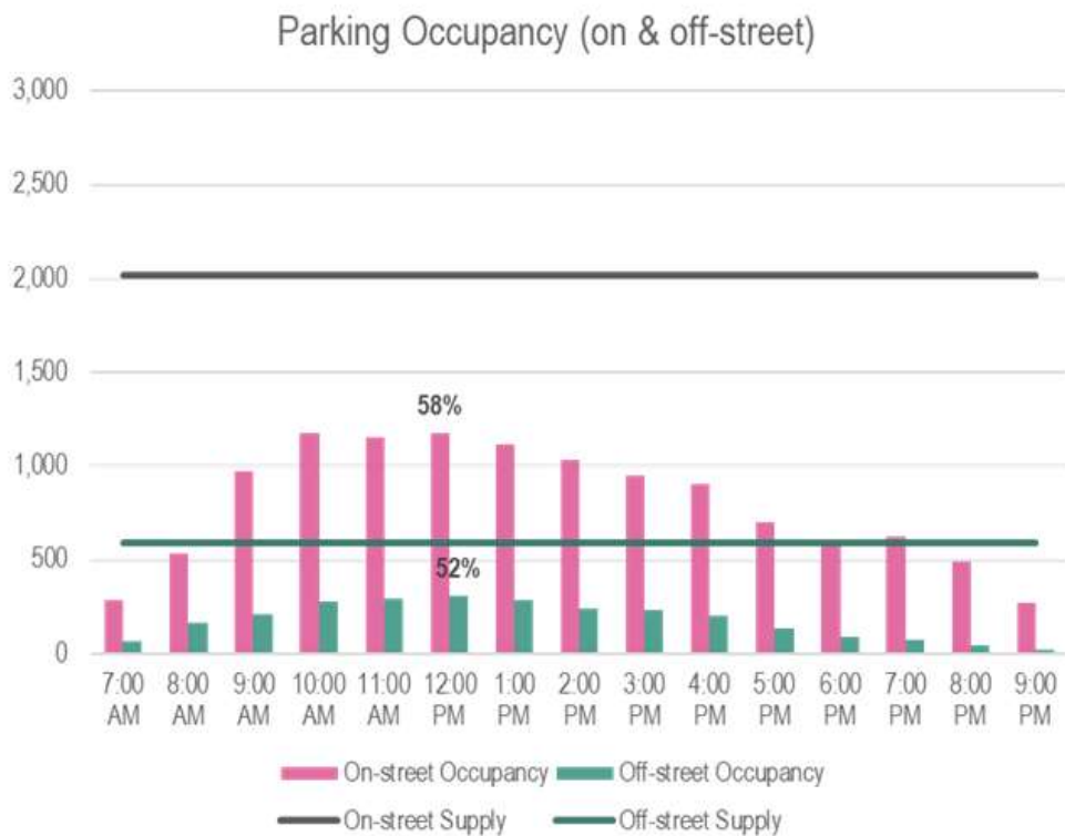
Figure 4: On-street and Off-street Parking Utilisation.
