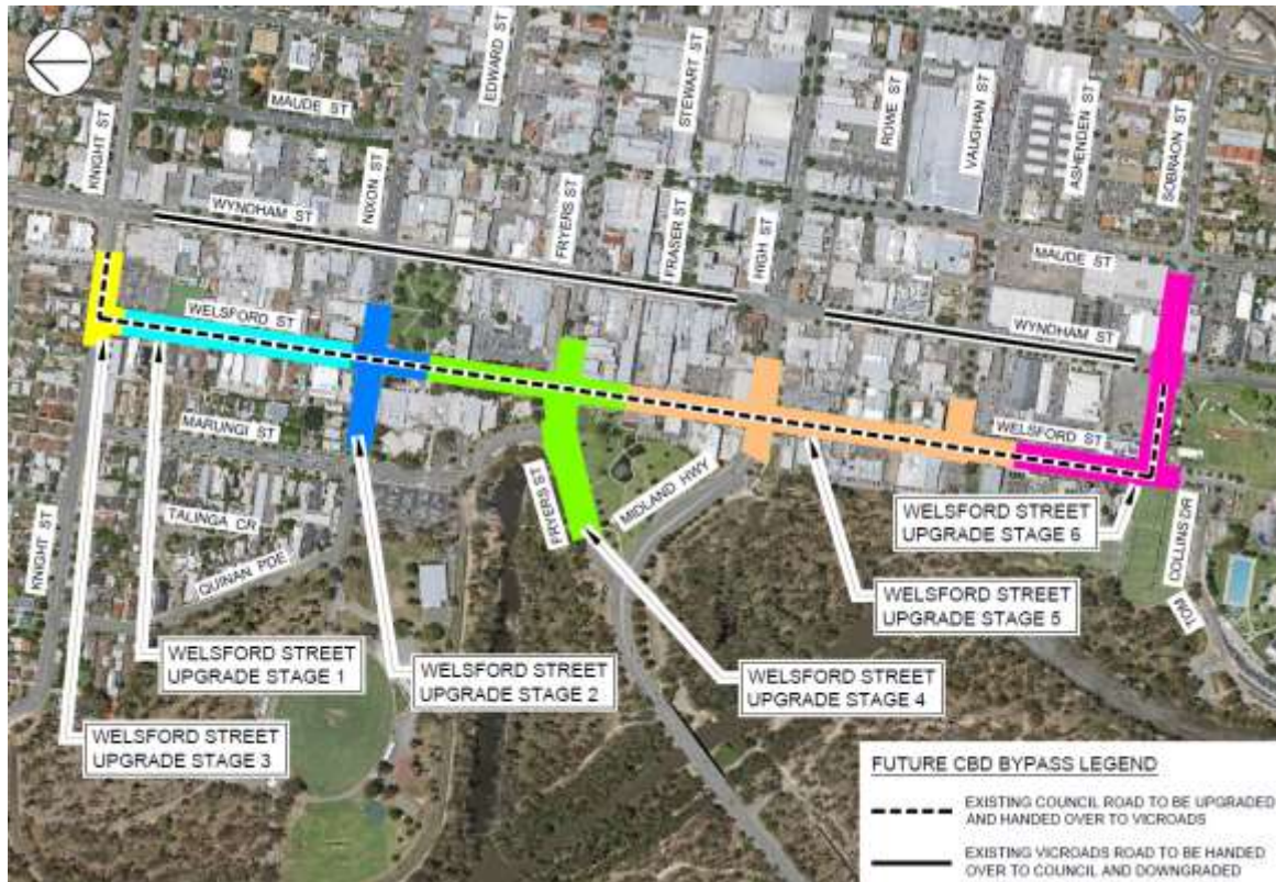
Figure 13: Welsford Street upgrade staging (Stages 1 to 3 are now complete).
